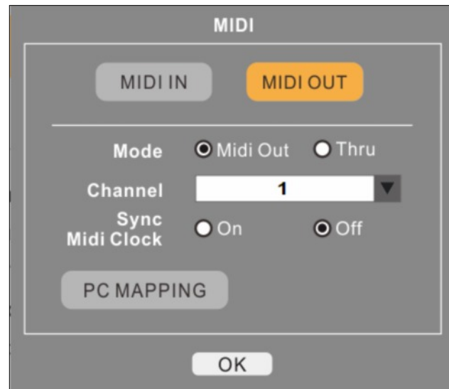
Figure 16 - The MIDI control box allows you to map MIDI channels to an external MIDI controller.
