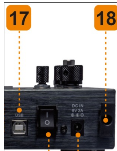
Figure 14 - The USB connection jack (17) is required to connect your PC to the Mooer Studio software and/or a DAW. Source: Mooer GE300 Owner's Manual.
