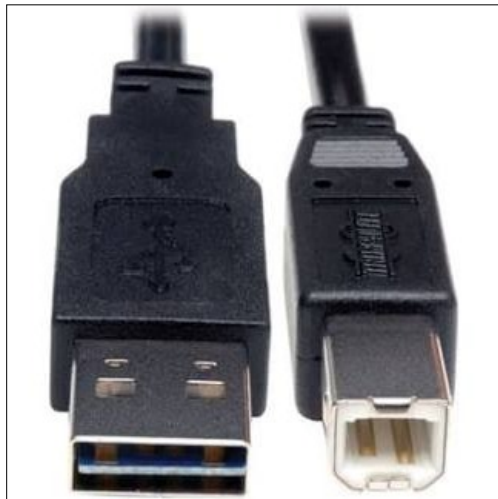
ABOVE LEFT: USB-A connection (to the PC) ABOVE RIGHT: USB-B connection (to the GE300 Unit)
